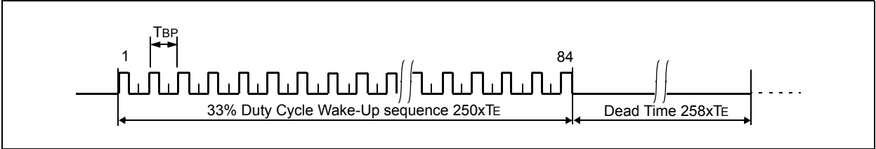
FIGURE 9-6: VPWM WAKE-UP FORMAT (MOD=1)
