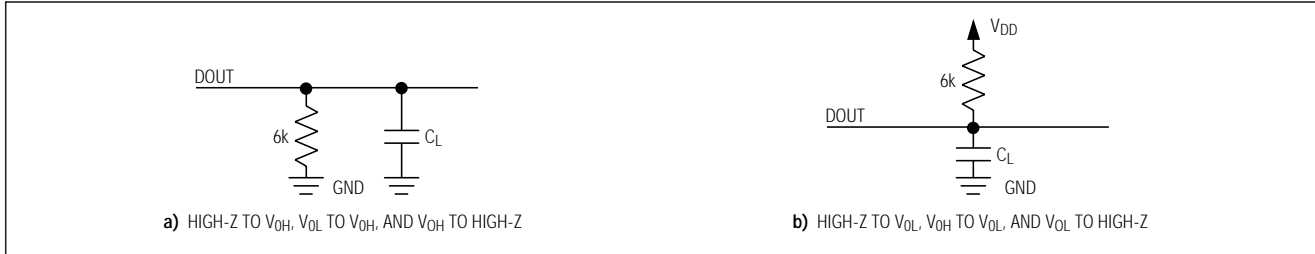
Figure 1. Load Circuits for Enable and Disable Time
