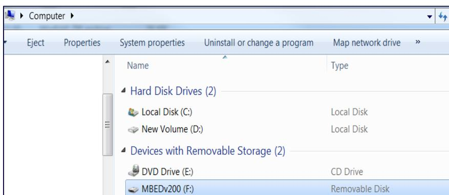
**Figure 2: Programming board appears as a flash drive**
