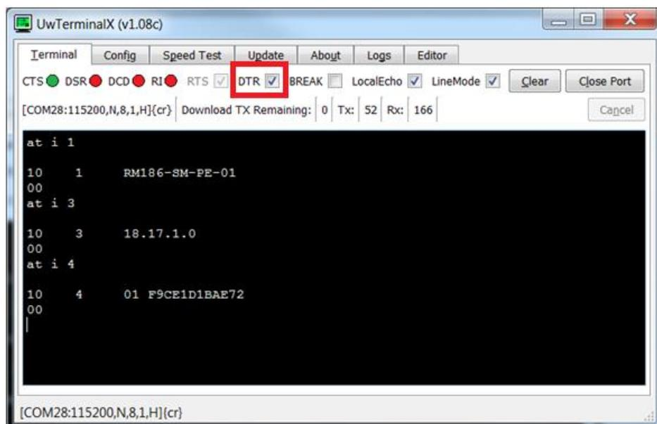
Figure 4: AT+I3 command returning the firmware version number
