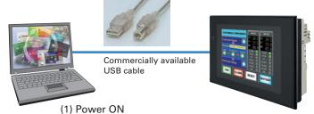
(2) Simply connect the USB cable and you are ready to transfer screen data and ladder programs.
