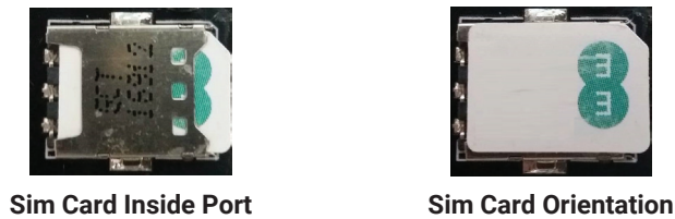
Figure 9 - Sim Card Orientation
