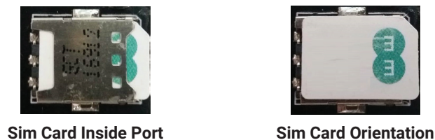
Figure 9 - Sim Card Orientation
