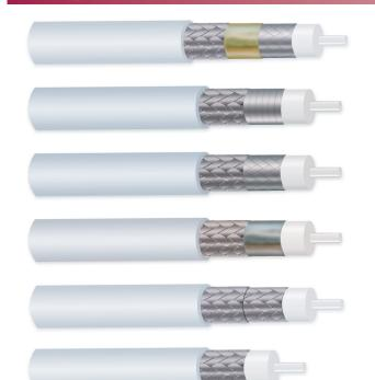
*Triple Shield* - Woven flat braid, polyemide foil, round braid. Provides >90 dB shielding effectiveness, high torque resistance, mechanically strong.
