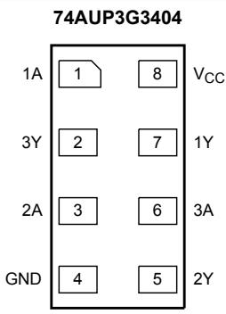
Fig. 5. Pin configuration SOT833-1, SOT1089, SOT1116 and SOT1203 (XSON8)
