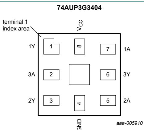
Fig. 6. Pin configuration SOT902-2 (XQFN8)
