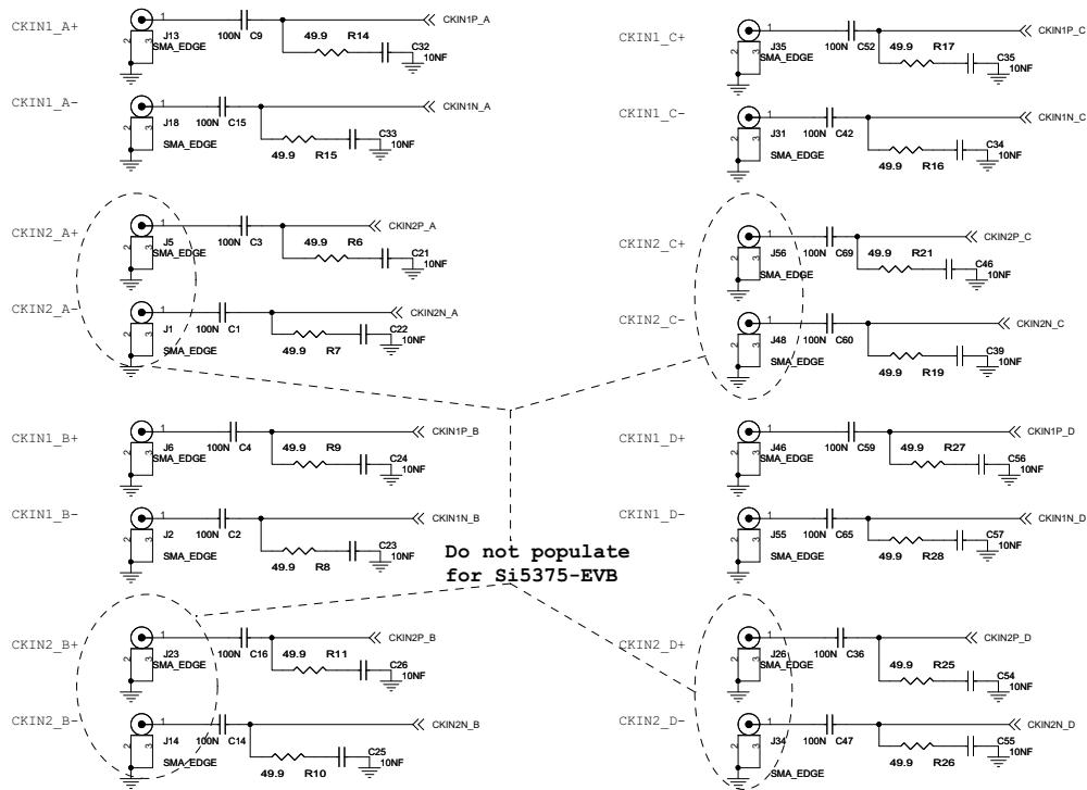
**Figure 5. Clock Inputs**
