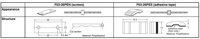
Note: The shape of the adhesive tape shown above is for securing the F03-16PE.
