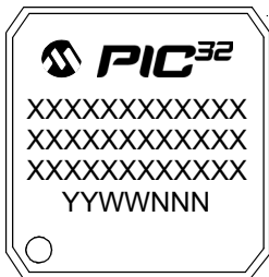
144-Lead TQFP (16x16x1 mm)
