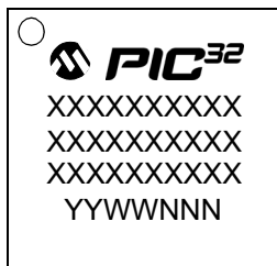
64-Lead QFN (9x9x0.9 mm)
