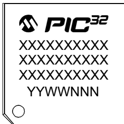
64-Lead TQFP (10x10x1 mm)
