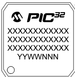
144-Lead TQFP (16x16x1 mm)
