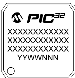
144-Lead TQFP (16x16x1 mm)
