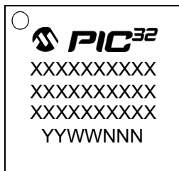
64-Lead QFN (9x9x0.9 mm)
