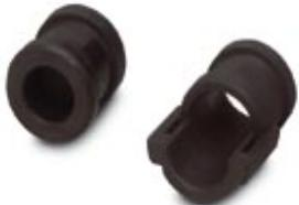
Cable feed-through sleeves, for cable diameters of 3 - 4 mm, a cable binder can be used as strain relief
