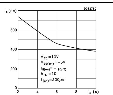
**Figure 12. Switching times resistive load**
