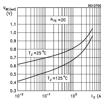
**Figure 7. Base-emitter on voltage**
