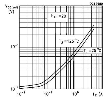
**Figure 5. Collector-emitter saturation voltage**
