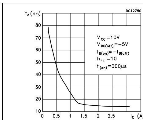
**Figure 11. Switching times inductive load**
