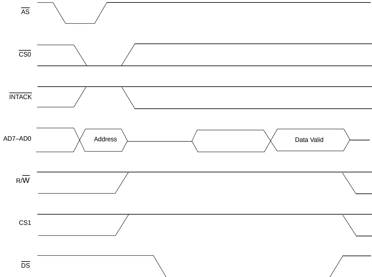
Figure 24. Read Cycle Timing
