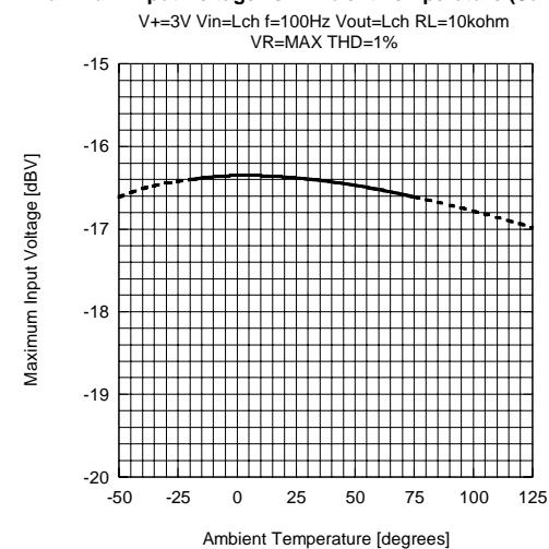
**Maximum Input Voltage vs. Ambient Temperature (BYPASS)**
