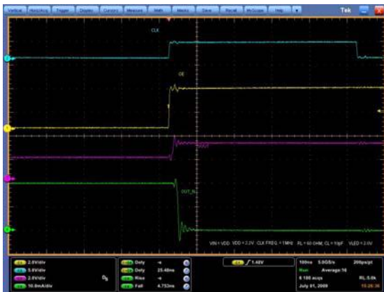
Figure 16: Turn ON output current characteristics (1)
