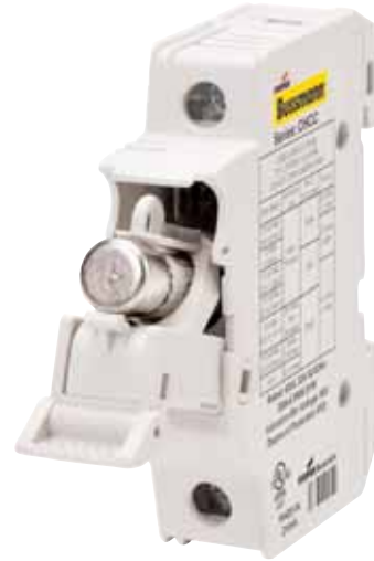
Series & Size Catalog Number Voltage & Current Agency Markings Number of Poles Terminal Rating SCCR Rating Cooper Bussmann Fuses With Indicator Without Indicator CHM 10x38 and Midget CHM1DIU CHM1DU UL 600V/30A; IEC 690V/32A cURus; IEC 60269-2 1 Solid, Stranded, Fine Stranded, Spade Lug, Comb Bus Bar; Single and Dual Wire; 75°C and 90°C Cu wire 100kA rms sym FNQ, KLM, FNM, KTK, BAF, FWA, DCM, C10 SERIES, AGU, BAN, FWC CHM2DIU CHM2DU 2 CHM3DIU CHM3DU 3 CHM4DIU CHM4DU 4 CHM1DNIU CHM1DNU UL 48Vdc/30A; IEC 48Vdc/32A IEC 60269-2 1 pole + 1 neutral n/a n/a CHM3DNIU CHM3DNU 3 poles + 1 neutral CHM1DI-48U 1 CHPV CHM1DNXU IEC 690V/32A IEC60269-2 1 neutral 75°C and 90°C Cu wire 33kA Solar PV series CHPV1IU CHPV1U UL & IEC; 1000Vdc/30A UR, CSA, UL4248-18, IEC60269-1 1 CHCC Class CC CHPV2IU CHPV2U 2 200kA rms sym LP-CC, FNQ-R, KTK-R CHCC1DIU CHCC1DU UL 600V/30A cULus 1 CHCC2DIU CHCC2DU 2 CHCC3DIU CHCC3DU 3 CHCC1DI-48U UL 48Vdc/30A 1
