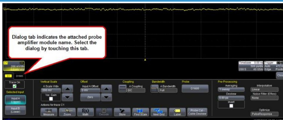
Vertical dialog with labeled tab corresponding with your attached probe.
