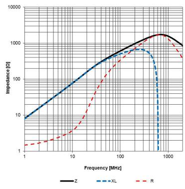
Test Equipment: E4991A or equivalent
