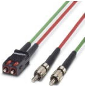
Assembled fiber optic cable, break-out cable, HCS fiber 200/230  $\mu\text{m}$ , SCRJ/IP20 on FSMA/IP20, for installation inside control cabinets, length: 2 m
