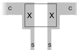
Note: Actual width of current trace is based on magnitude of current. Point of connection should be in the area shown.
