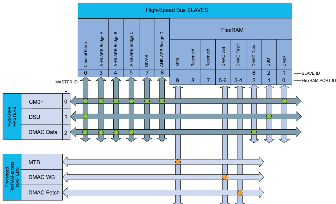
Figure 11-1. Master-Slave Relation High-Speed Bus Matrix (1)
