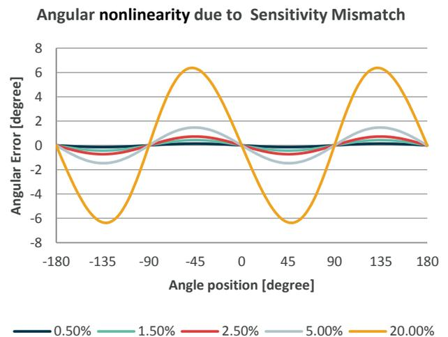
Figure 23: Angle nonlinearity due to sensitivity Mismatch
