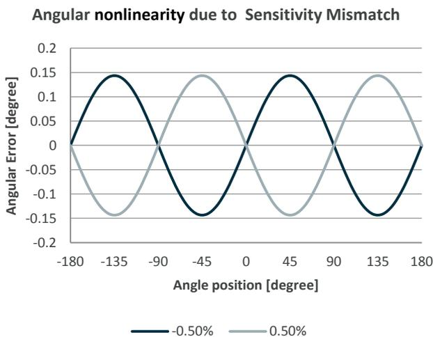
Figure 22: Angle nonlinearity due to sensitivity Mismatch
