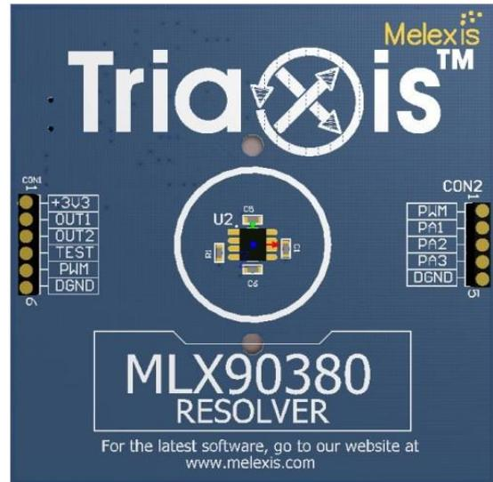
*Figure 1: MLX90380 Resolver Evaluation/Demonstration board*
