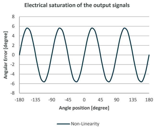
Figure 25: Angle nonlinearity due to signal saturation.
