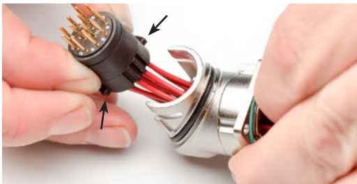
Step 5 - Locate keys on sides of insert
