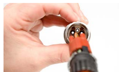
Step 14 - Trim shield as shown
