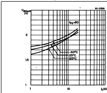
**Figure 9. Base-emitter saturation voltage**
