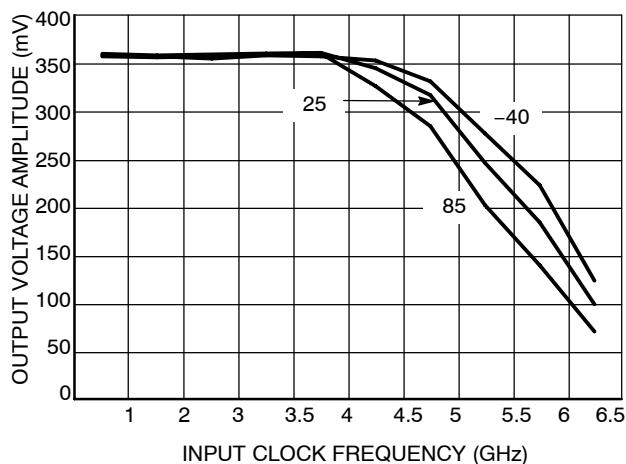
**Figure 4. Output Voltage Amplitude vs. Input Clock Frequency and Temperature**
