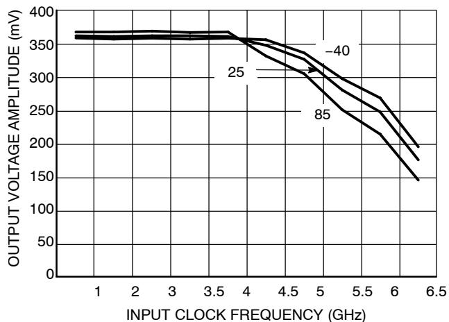
**Figure 3. Output Voltage Amplitude vs. Input Clock Frequency and Temperature**
