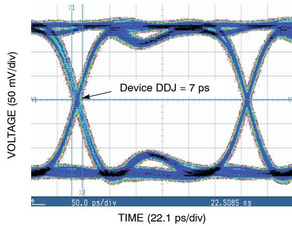
**Figure 8. Typical Output Waveform at 3.125 Gb/s with PRBS 2<sup>23</sup>-1 ( $V_{inpp} = 75 \text{ mV-left and } 400 \text{ mV-right}$ )**
