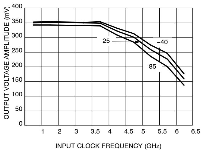
**Figure 5. Output Voltage Amplitude vs. Input Clock Frequency and Temperature**
