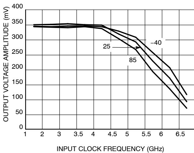
**Figure 6. Output Voltage Amplitude vs. Input Clock Frequency and Temperature**
