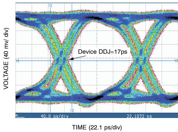
**Figure 9. Typical Output Waveform at 5 Gb/s with PRBS 2<sup>23</sup>-1 ( $V_{inpp}=75 \text{ mV-left and } 400 \text{ mV-right}$ )**
