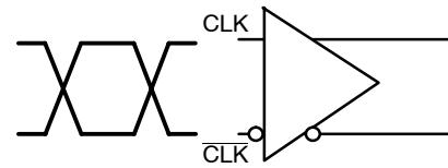
**Figure 14. Differential Inputs Driven Differentially**
