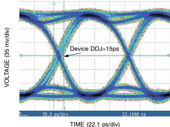
**Figure 10. Typical Output Waveform at 6.125 Gb/s with PRBS 2<sup>23</sup>-1 ( $V_{inpp} = 75 \text{ mV-left and } 400 \text{ mV-right}$ )**
