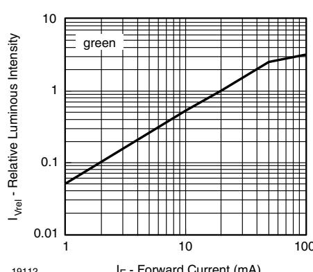
Fig. 23 - Relative Luminous Intensity vs. Forward Current
