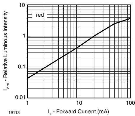
Fig. 33 - Relative Luminous Intensity vs. Forward Current
