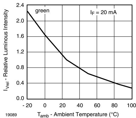
Fig. 20 - Relative Luminous Intensity vs. Ambient Temperature
