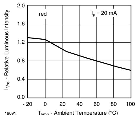
Fig. 30 - Relative Luminous Intensity vs. Ambient Temperature
