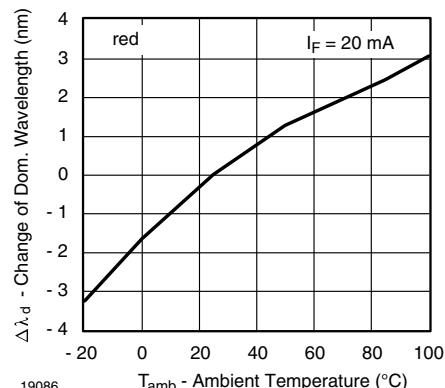
Fig. 29 - Change of Dominant Wavelength vs. Ambient Temperature
