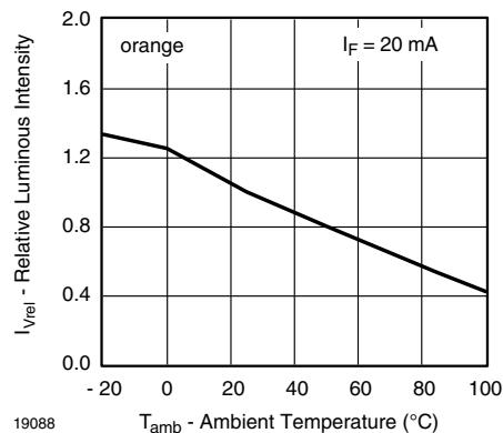
Fig. 3 - Relative Luminous Intensity vs. Ambient Temperature
