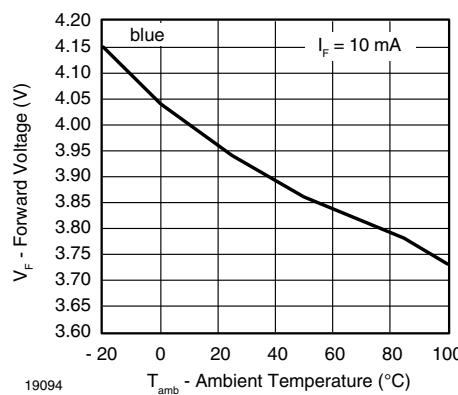
Fig. 11 - Forward Voltage vs. Ambient Temperature
