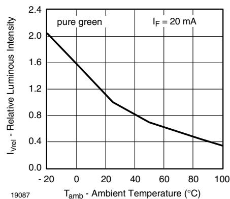
Fig. 15 - Relative Luminous Intensity vs. Ambient Temperature
