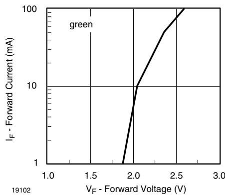
Fig. 22 - Forward Current vs. Forward Voltage
