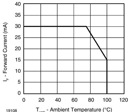
Fig. 1 - Forward Current vs. Ambient Temperature
