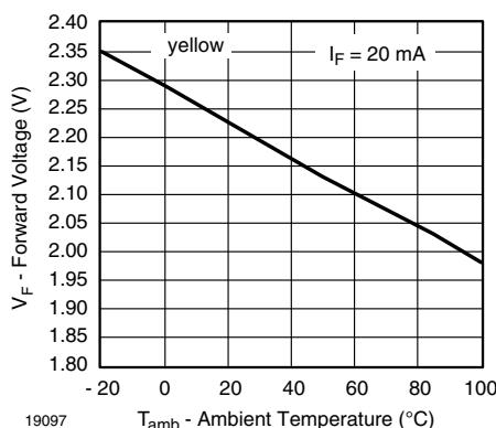
Fig. 26 - Forward Voltage vs. Ambient Temperature
