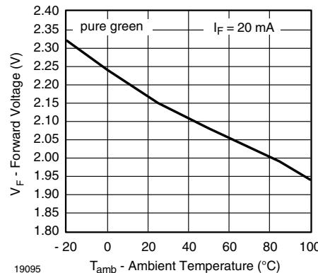
Fig. 16 - Forward Voltage vs. Ambient Temperature
