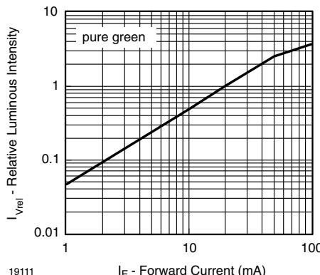
Fig. 18 - Relative Luminous Intensity vs. Forward Current
