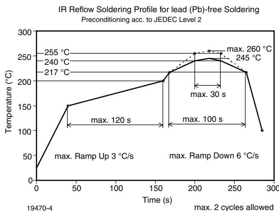
Fig. 34 - Vishay Lead (Pb)-free Reflow Soldering Profile
