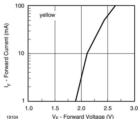
Fig. 27 - Forward Current vs. Forward Voltage
