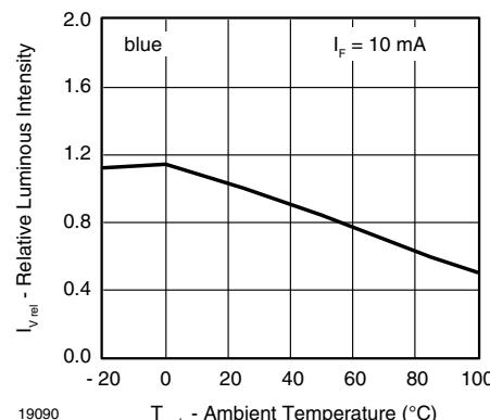
Fig. 10 - Relative Luminous Intensity vs. Ambient Temperature
