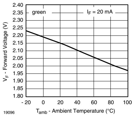
Fig. 21 - Forward Voltage vs. Ambient Temperature
