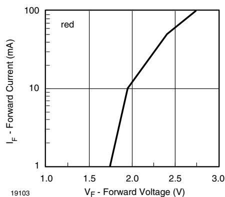
Fig. 32 - Forward Current vs. Forward Voltage
