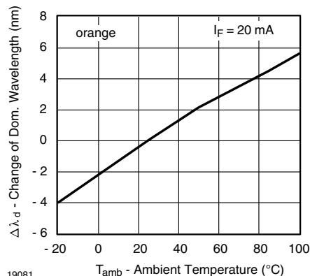
Fig. 2 - Change of Dominant Wavelength vs. Ambient Temperature
