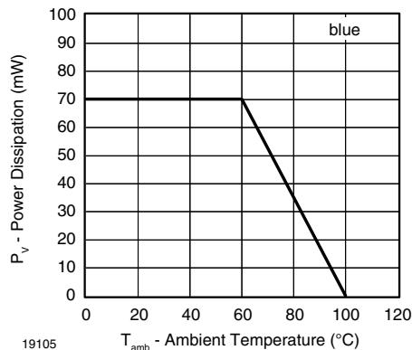
Fig. 7 - Power Dissipation vs. Ambient Temperature
