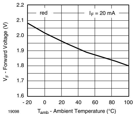
Fig. 31 - Forward Voltage vs. Ambient Temperature
