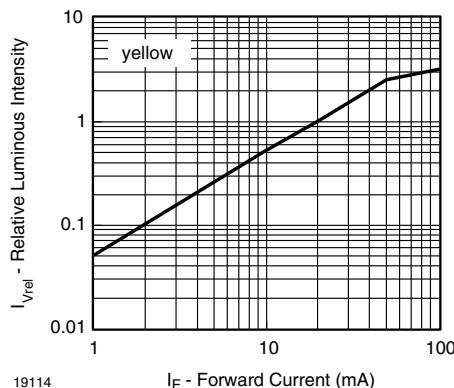
Fig. 28 - Relative Luminous Intensity vs. Forward Current
