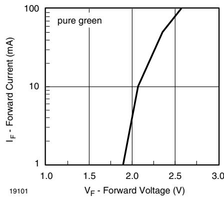
Fig. 17 - Forward Current vs. Forward Voltage
