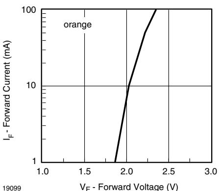
Fig. 5 - Forward Current vs. Forward Voltage
