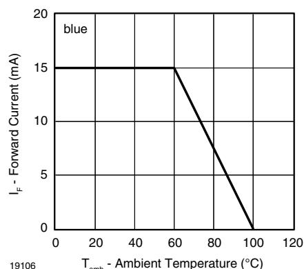
Fig. 8 - Forward Current vs. Ambient Temperature
