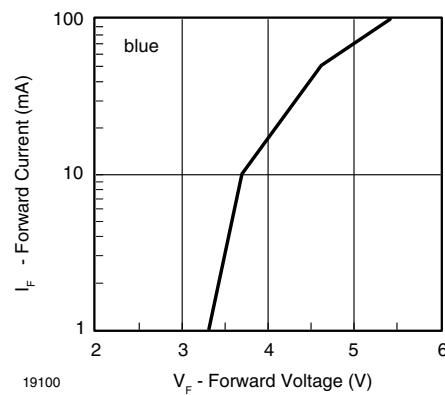
Fig. 12 - Forward Current vs. Forward Voltage
