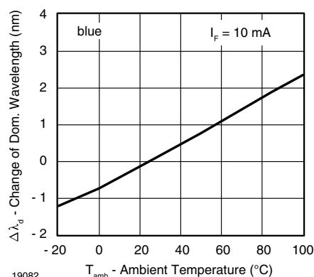
Fig. 9 - Change of Dominant Wavelength vs. Ambient Temperature
