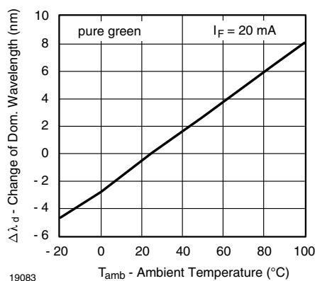
Fig. 14 - Change of Dominant Wavelength vs. Ambient Temperature
