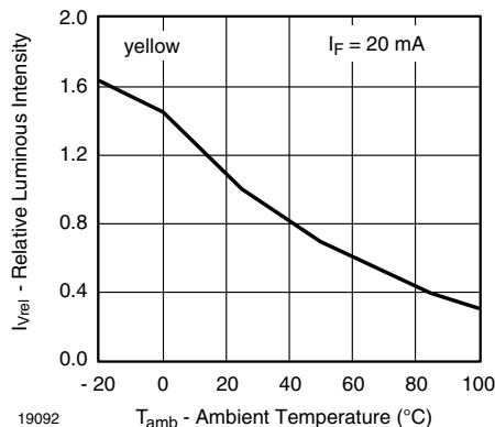
Fig. 25 - Relative Luminous Intensity vs. Ambient Temperature
