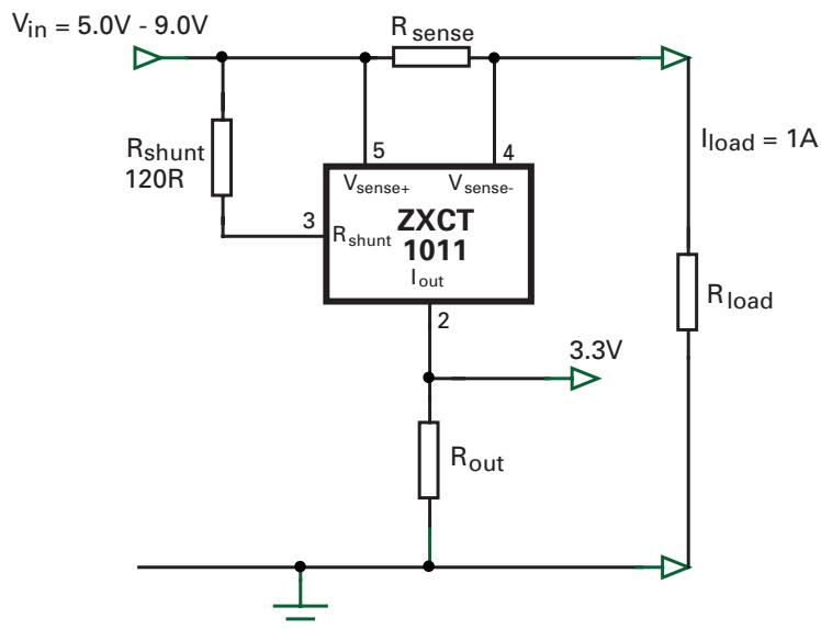
**Figure 1 ZXCT1011 to measure a 1.0 A load current**
