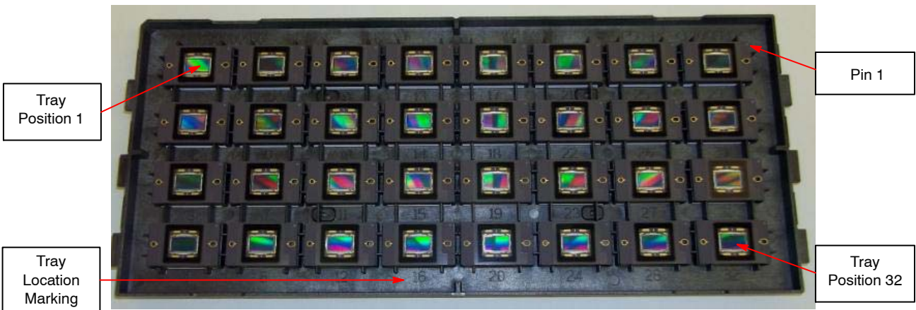
Figure 35. Tray Pin-Down View
