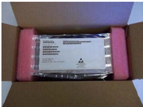
Figure 39. Brick Loaded in Shipping Container
