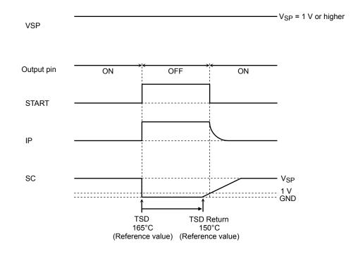
Note: The TSD circuit is not intended to provide protection against all abnormal conditions. Therefore, the TB6588FG should exit the abnormal state immediately after the TSD circuit is enabled. If the device is used beyond the absolute maximum ratings, the TSD circuit may not operate properly, or the device may break down before the protection circuit is activated.
