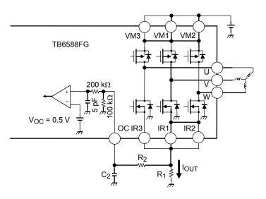
Note: The overcurrent protection circuit (normally a current limiter) is not intended to provide protection against all abnormal conditions. Therefore, the TB6588FG should exit the abnormal state immediately after the overcurrent protection circuit is enabled.
