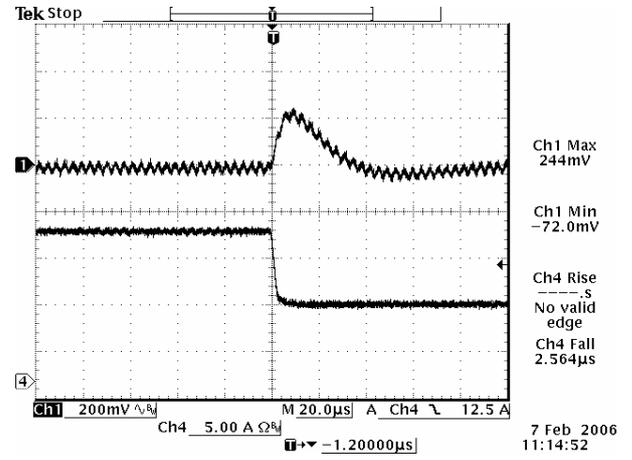
100% to 50% load Transient at 5.0 Vdc output
