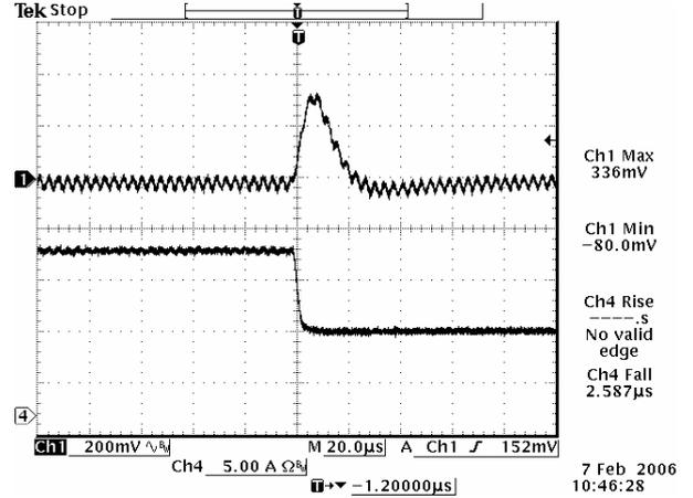
100% to 50% load Transient at 5.0 Vdc output
