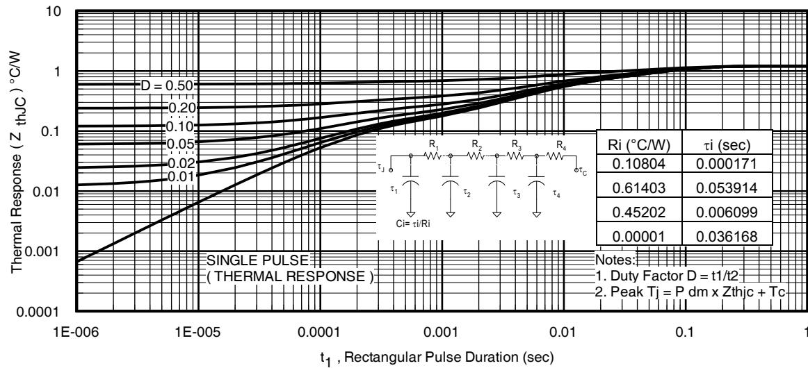
**Fig 15.** Maximum Effective Transient Thermal Impedance, Junction-to-Case
