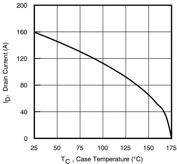
Fig 12. Maximum Drain Current vs. Case Temperature
