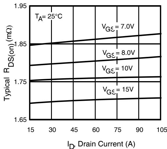
**Fig. 4** Typical On-Resistance vs. Drain Current
