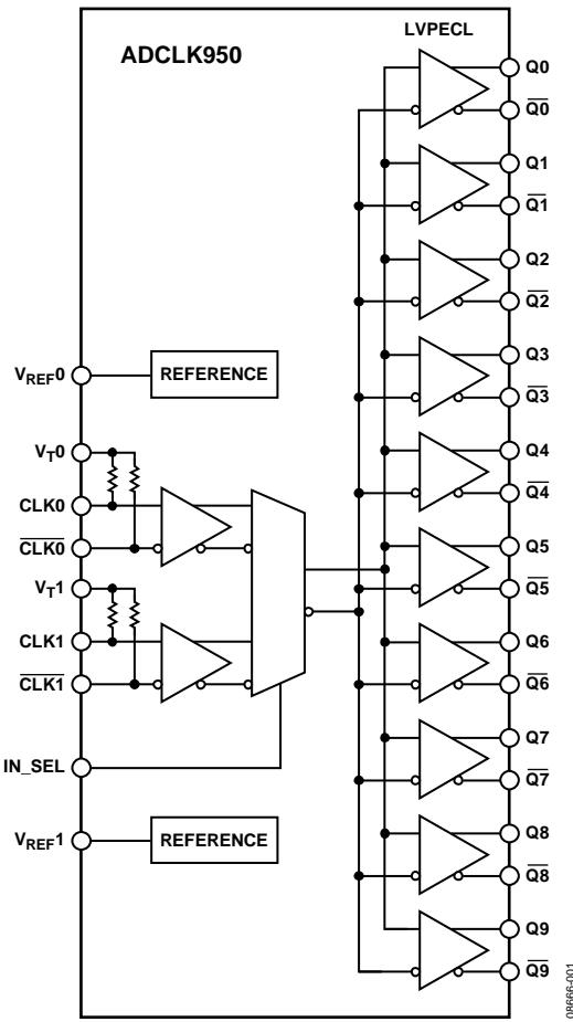
Figure 3. ADCLK950 1:10 Clock/Data Buffer Block Diagram
