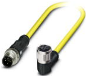
Sensor/Actuator cable, 4-position, PVC, Yellow RAL 1021, Plug straight M12-SPEEDCON, A-coded, on Socket angled M12-SPEEDCON, A-coded, Cable length: 0.5 m
