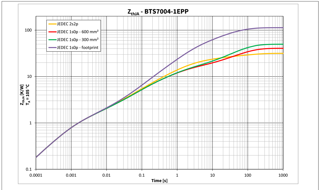
Figure 9 Typical Thermal Impedance. PCB setup according Chapter 4.4.1
