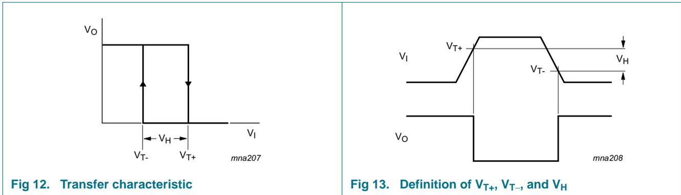
Fig 12. Transfer characteristic
