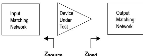
**Figure 13. Series Equivalent Source and Load Impedance**
