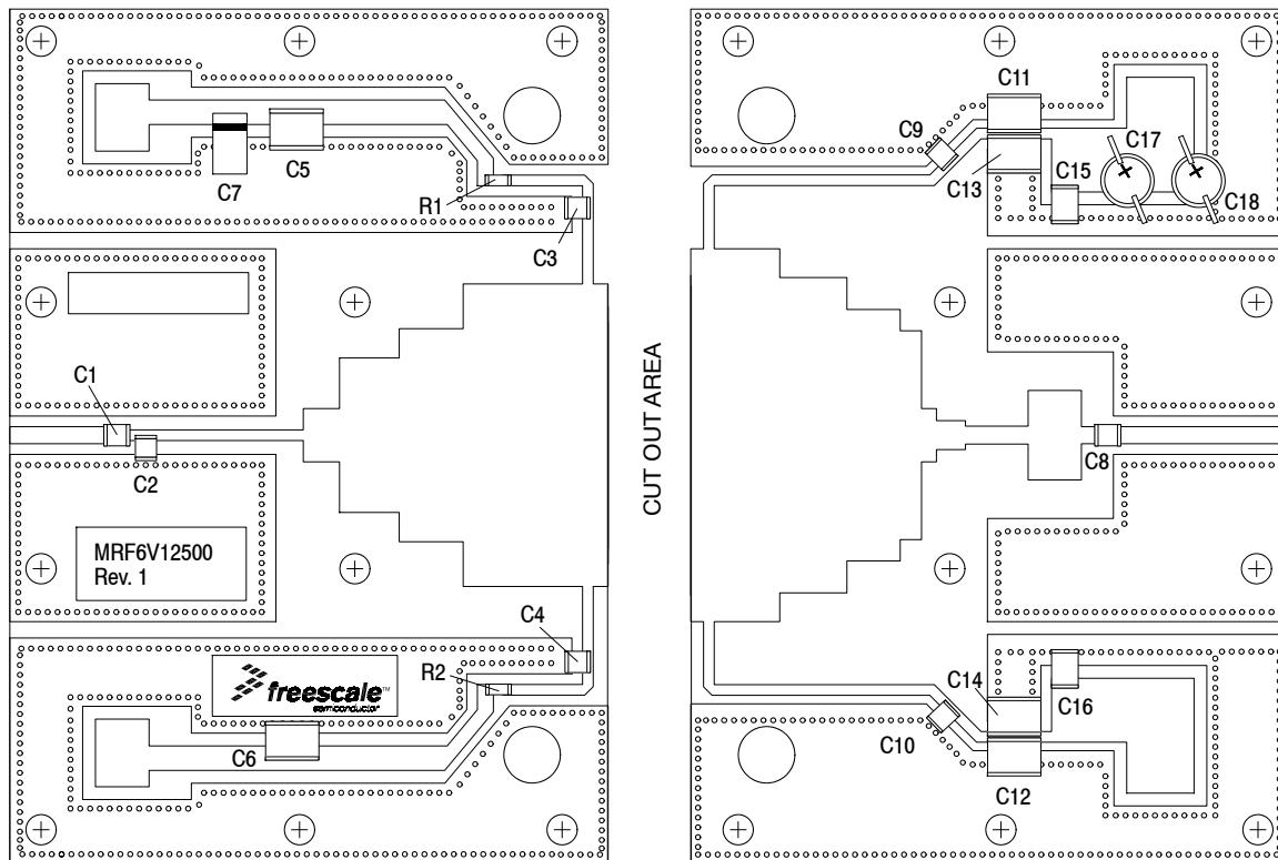
**Figure 14. MRF6V12500H(HS) Test Circuit Component Layout — 960-1215 MHz**
