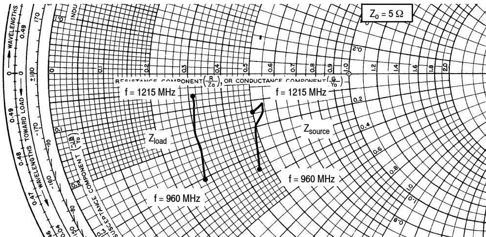
$V_{DD} = 50 \text{ Vdc}$ ,  $I_{DQ} = 200 \text{ mA}$ ,  $P_{out} = 500 \text{ W Peak}$
