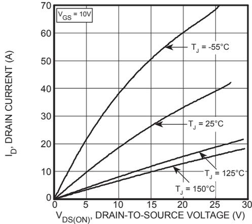
Figure 1, Output Characteristics
