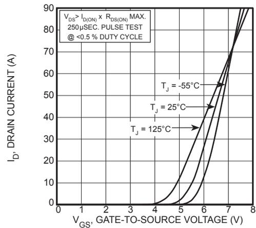
Figure 4, Transfer Characteristics
