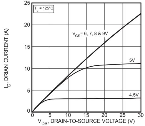
Figure 2, Output Characteristics
