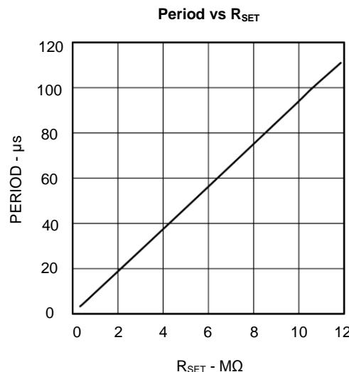
Figure 2. FOUT/PWMOUT Period vs  $R_{SET}$
