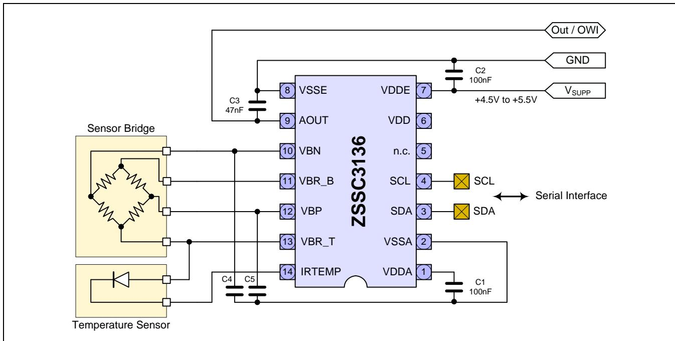
**Figure 3.3 Application with External Thermistor**
