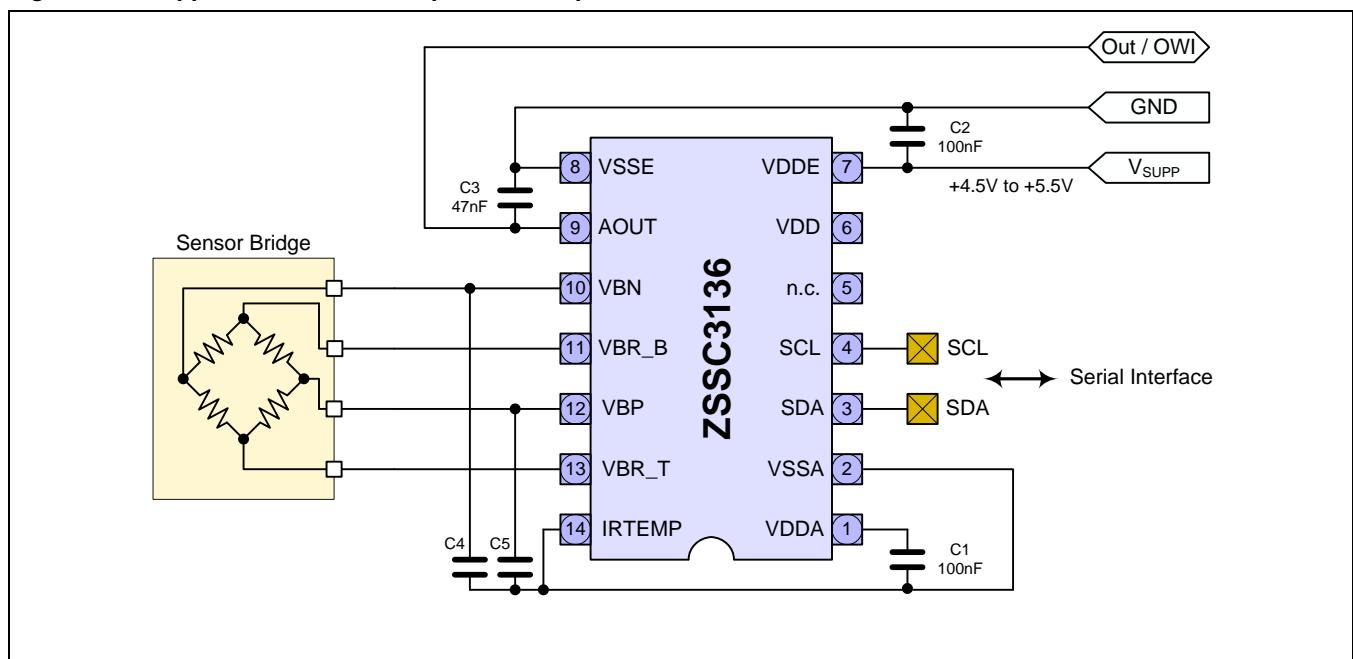
**Figure 3.2 Application with External Diode Temperature Sensor**
