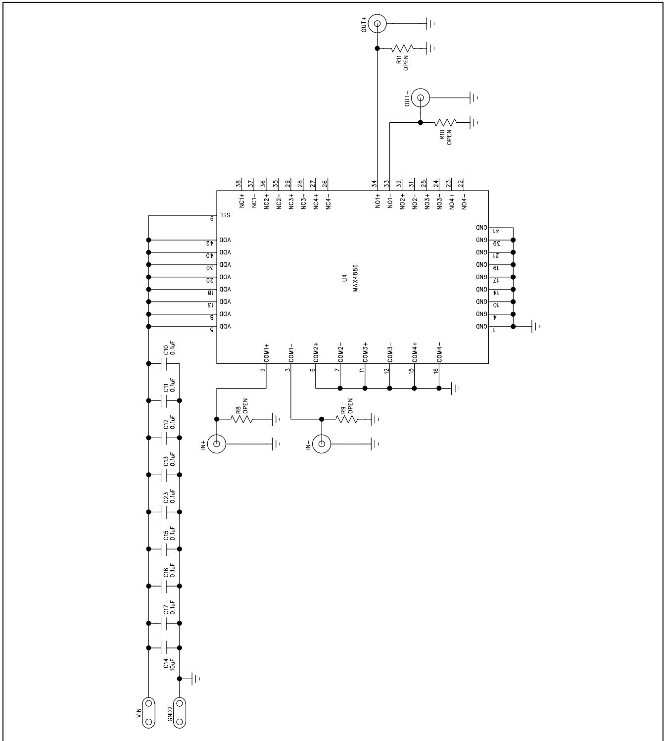
Figure 1b. MAX4886 EV Kit Schematic (Sheet 2 of 2)
