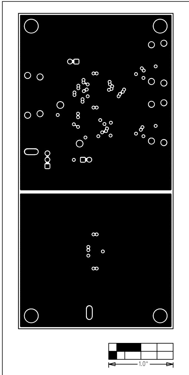
Figure 4. MAX4886 EV Kit PCB Layout—GND Layer 2
