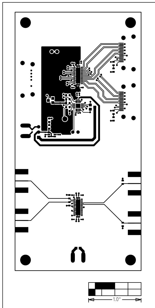
Figure 3. MAX4886 EV Kit PCB Layout—Component Side
