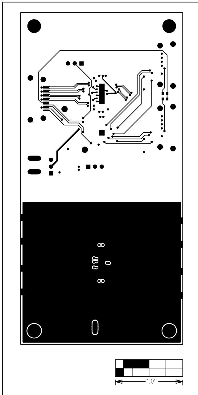
*Figure 6. MAX4886 EV Kit PCB Layout—Solder Side*
