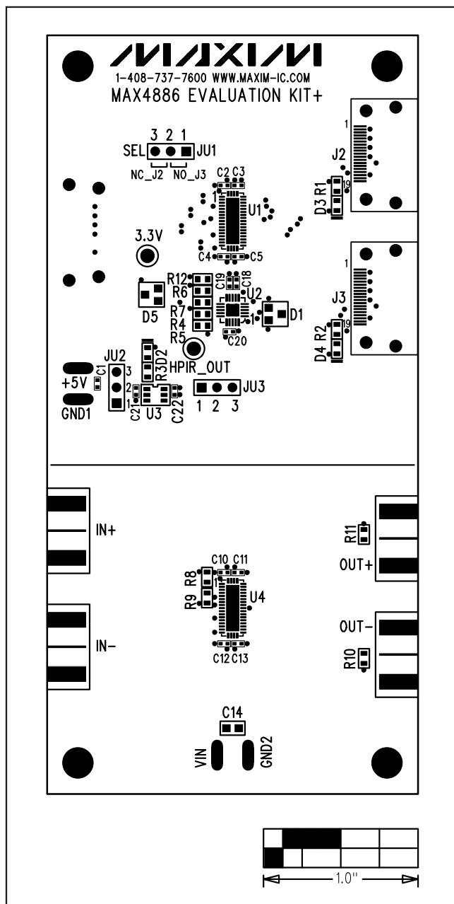
Figure 2. MAX4886 EV Kit Component Placement Guide—Top Silkscreen
