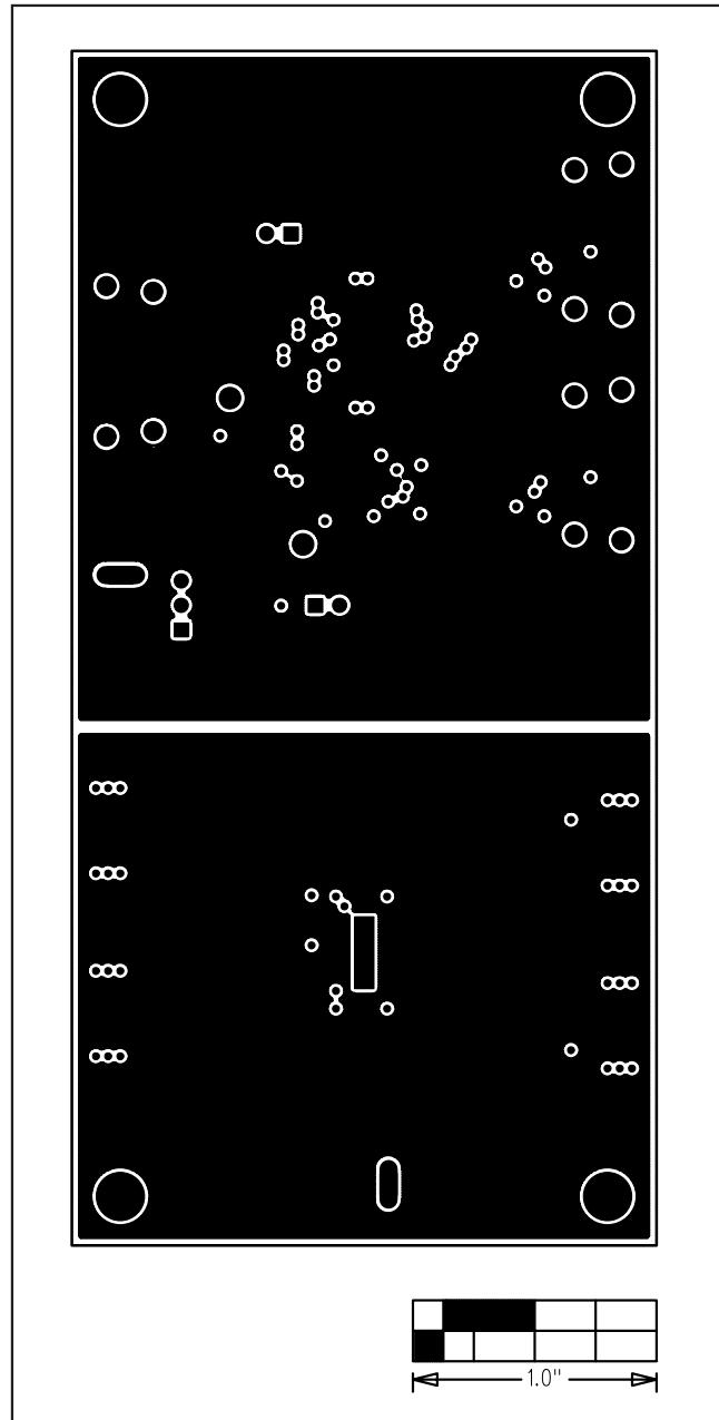
Figure 5. MAX4886 EV Kit PCB Layout—GND Layer 3
