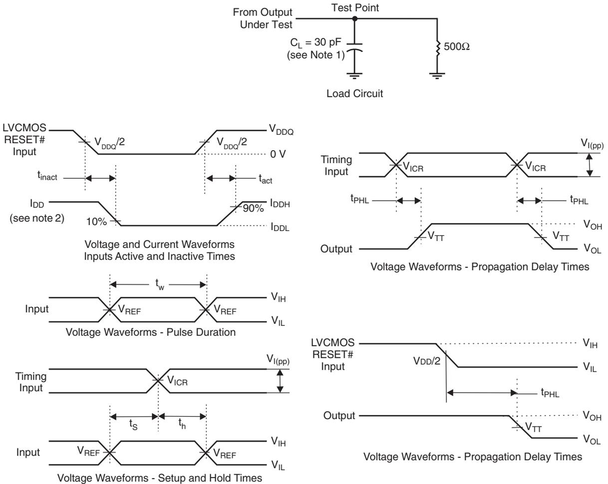
Figure 1 - Parameter Measurement Information ( $V_{DDQ} = 2.5V \pm 0.2V$ )
