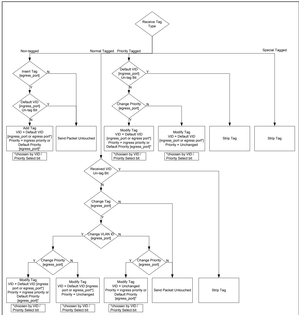
FIGURE 10-7: HYBRID PORT TAGGING AND UN-TAGGING
