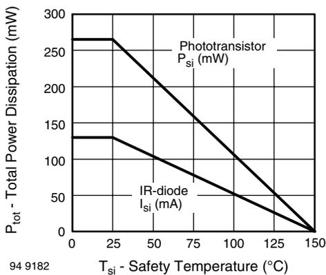
Fig. 1 - Derating Diagram
