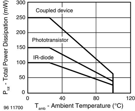
Fig. 6 - Total Power Dissipation vs. Ambient Temperature
