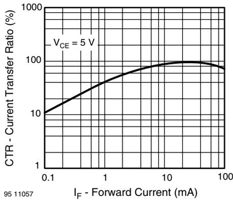
Fig. 12 - Current Transfer Ratio vs. Forward Current
