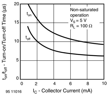
Fig. 14 - Turn-on/off Time vs. Collector Current
