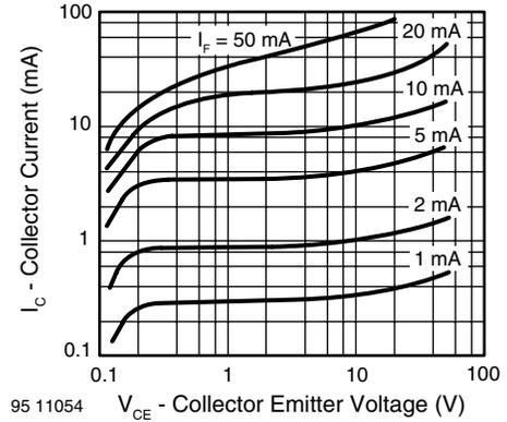
Fig. 10 - Collector Current vs. Collector Emitter Voltage
