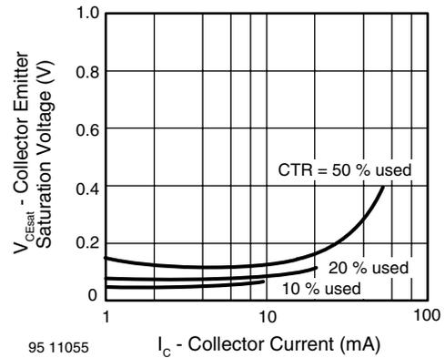
Fig. 11 - Collector Emitter Saturation Voltage vs. Collector Current
