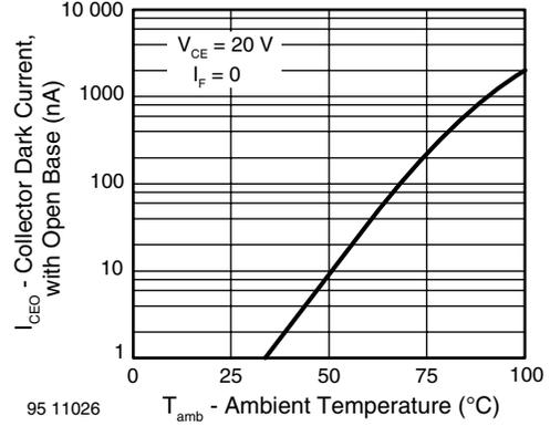
Fig. 9 - Collector Dark Current vs. Ambient Temperature
