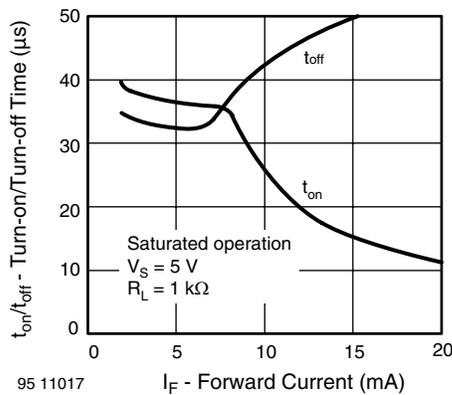
Fig. 13 - Turn-on/off Time vs. Forward Current
