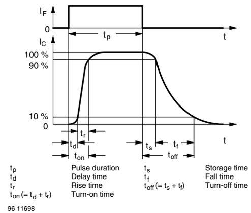
Fig. 5 - Switching Times
